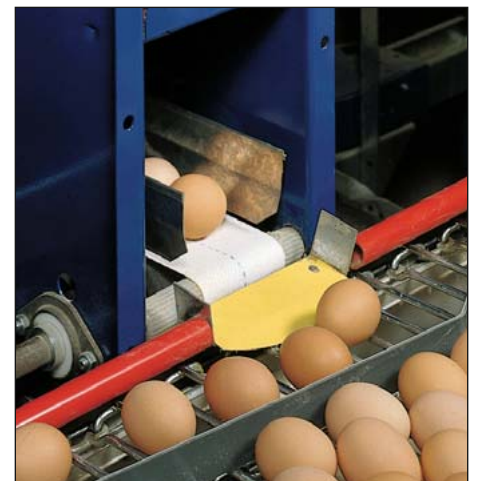
Egg transfer from longitudinal belt to cross belt
