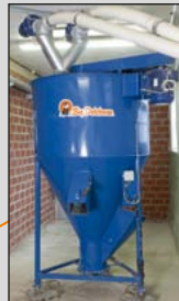
Day hopper with mixing function
