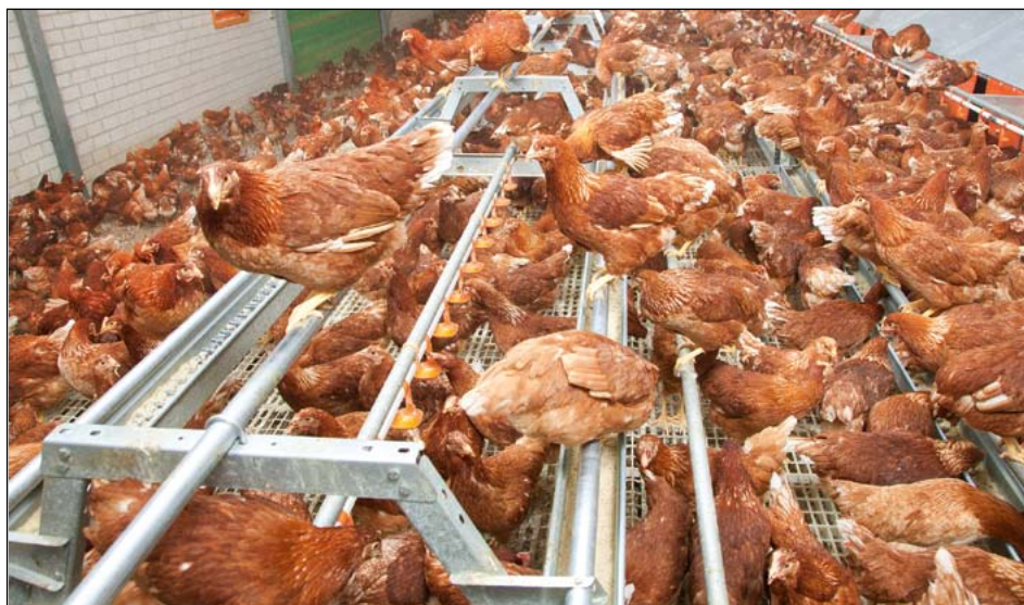
A-frame 5800 with 6 perches, two feed lines and a water line
