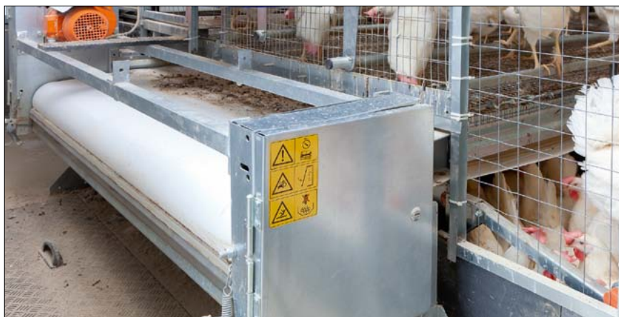
Manure belt beneath the supply zone in the one-tier NATURA-Nova
