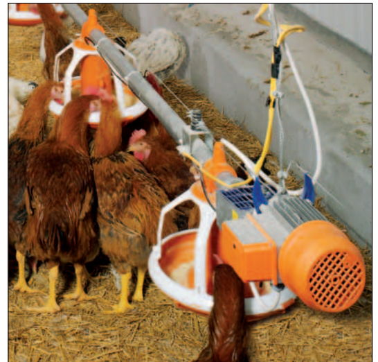
AUGERMATIC system with MALE PAN and Rapid Rooster drive for separate male feeding
