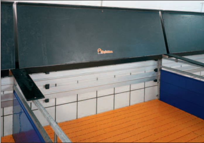
Underneath the covering plate, plastic flooring with 10 % slatted area is used; twin pipes ensure optimum temperatures in the resting area
