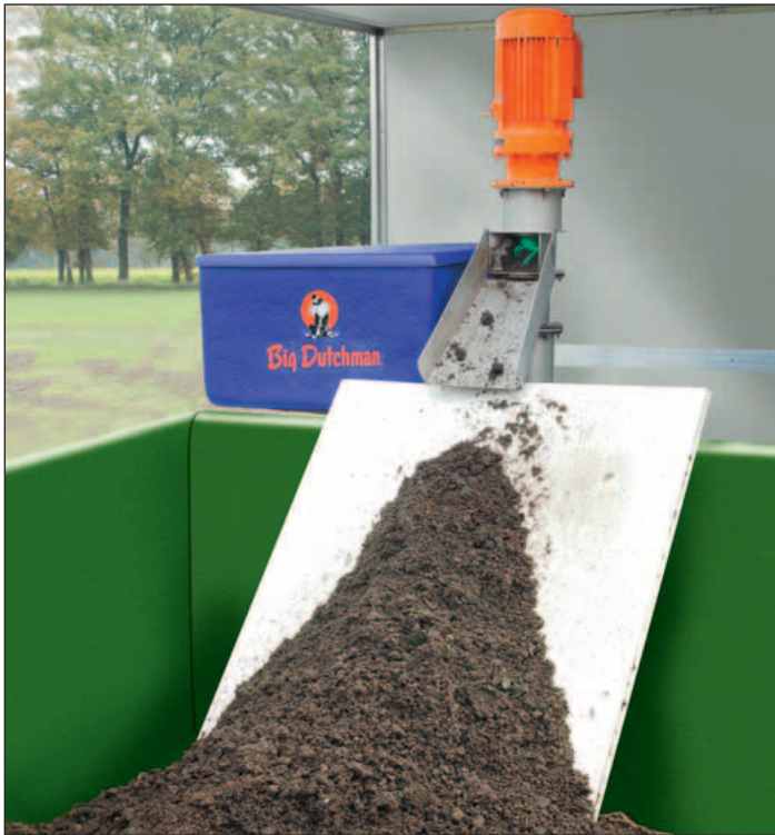
OptiPress I for materials with a low dry matter content and a homogenous structure (ie. of even particle size)
