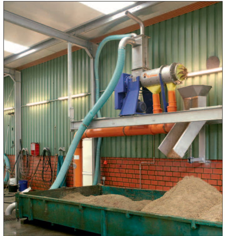
OptiPress II for materials with increased dry matter content and a more coarse structure
